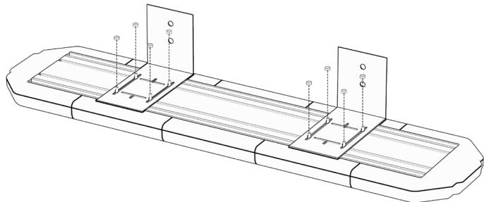
NOTE: IT IS VERY IMPORTANT TO POSITION THE BRACKET SO THAT THE LONGER PART OF BRACKET THAT ATTACHES TO THE LIGHTBAR POINTS TO THE REAR OF THE VEHICLE.
